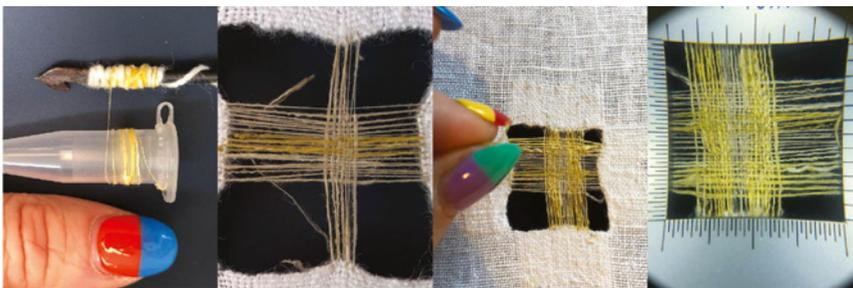
**Figure 29.3** Spinning and weaving spider silk. Source: Image credit Flanagan ©2021.
