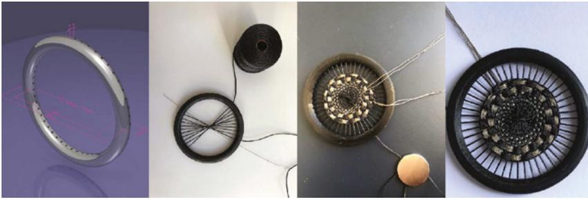
**Figure 29.8** Plant bio-electro-physiological mouthring speaker prototype. Source: Image credit Flanagan ©2021.
